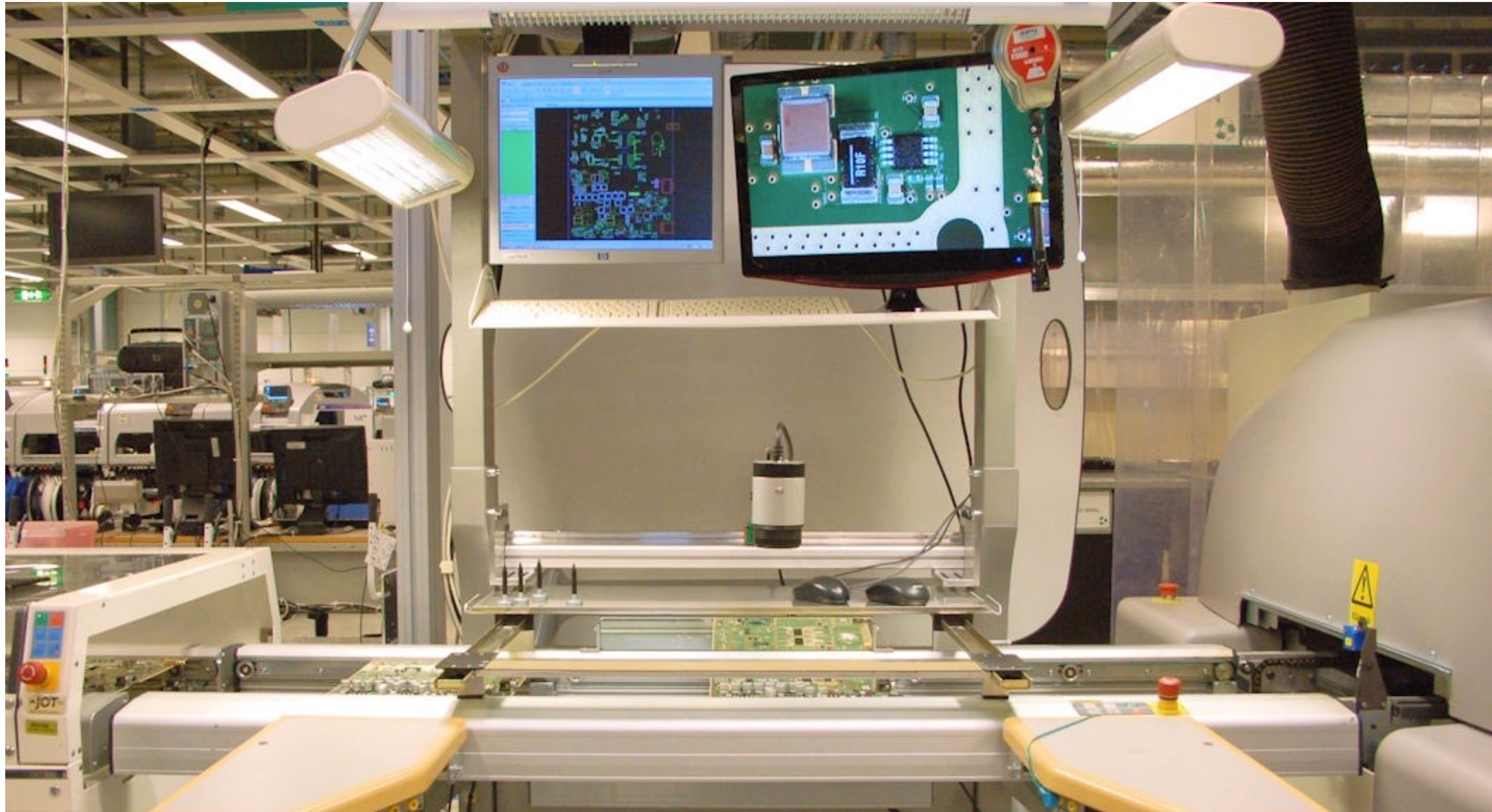
The Camera positioned over conveyor after Pick & Place
